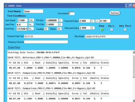
The FAT test screen reports the test conditions and provides a tabular listing of the test results during the execution of the test sequence.
