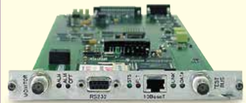
Backplane Interface Card (BIF) is installed in a dedicated card slot in the 28000 mainframe.
