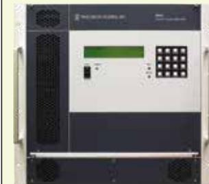
**Computer-controlled analog signal switching replaces tedious manual patch panels.**
