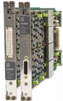
28304 with Auxiliary Output Connector, left, and the 28304 with Option 4, right
