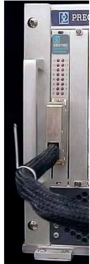
28316C Card Installed in 28016-M3 Frame
