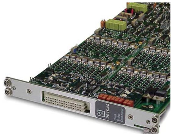
28104A Front Panel with Auxiliary Output Connector
