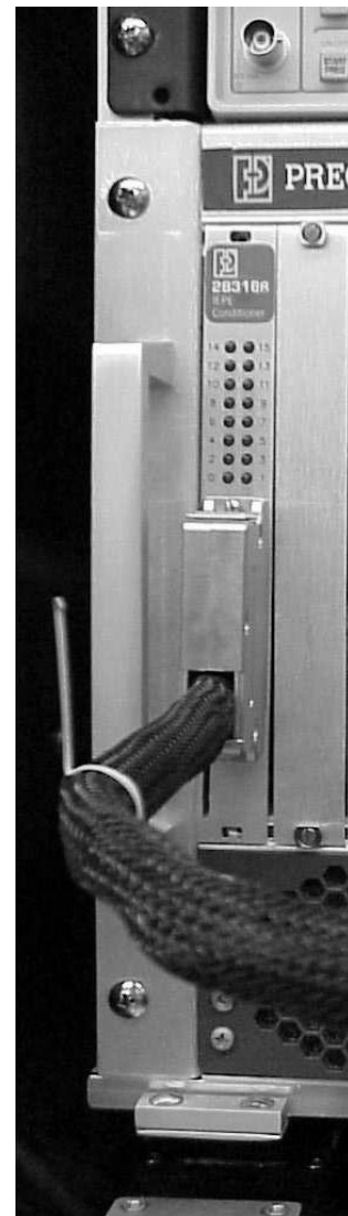
28316A Card Installed in 28016-M3 Frame
