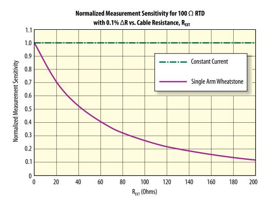
Figure 2: Normalized Measurement Sensitivity vs. R<sub>EXT</sub>
