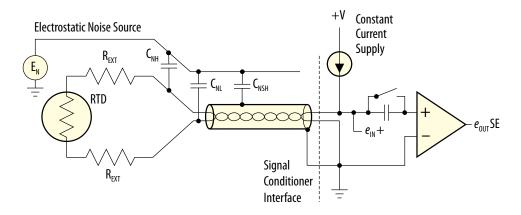
Figure 3: Single-Ended Constant Current Excitation Circuit
