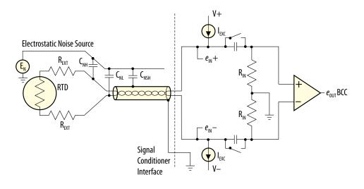
**Figure 4:** Balanced Constant Current Excitation Circuit
