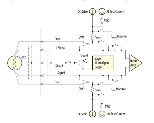
Figure 5: Balanced Constant Current Excitation Circuit Diagram
