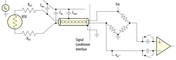
Figure 1: Two-Wire Wheatstone Bridge Connection
