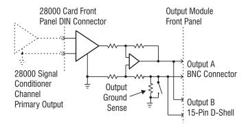
Figure 2 BUFF-4BNC/15D Channel Diagram (1 of 4 Channels)
