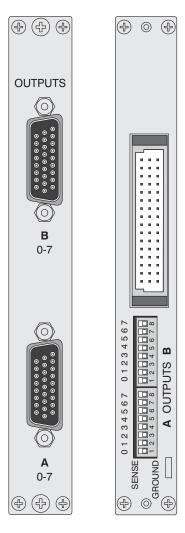
Figure 5 BUFF-8CH/(2)HD26D Dual Buffer Front and Rear Panels
