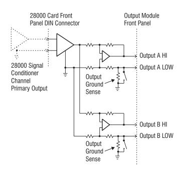
Figure 4 Channel Block Diagram for the BUFF-4CH/(2)15D and the BUFF-8CH/(2)HD26D Dual Buffer Modules
