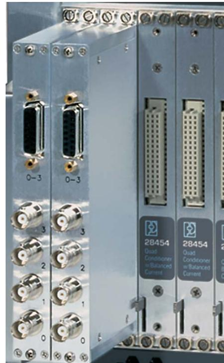
Figure 1 BUFF-4BNC/15D Output Buffer Modules
