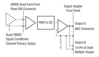
28000-RMS/DC4 Channel Diagram (1 of 4 Channels)
