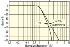
The input to output time delay of the LP6F and Butterworth are not constant versus frequency as a consequence of the non-linear phase property of these filters. Filters with linear phase, such as the Precision LP6P, have linear phase and thus constant delay for all frequencies in the pass-band.
