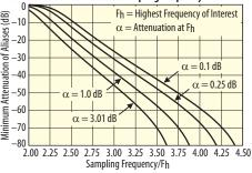
In exchange for linear phase and excellent transient response, the LP6P is less selective and thus requires a higher sampling frequency than the LP6F.
