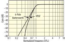
Band-Pass Amplitude Response HP6F and LP6F Cascaded
