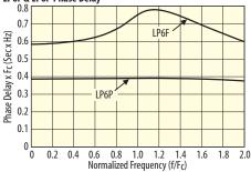
When compared to a 6-pole Bessel filter, the LP6P has similar pass-band characteristics yet has much sharper transition slope from pass-band to stop-band.
