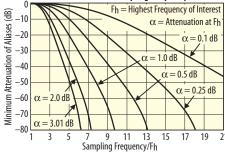
The chart below provides a comparison of attenuation of aliases versus sampling frequency for the LP6P, 6-pole Bessel (BE6), LP6F and the 6-pole Butterworth (BU6). It is clear that much lower sampling frequencies are required for the Precision LP6P and LP6F when compared to traditional filter characteristics.
