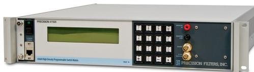
The built-in Go/No-Go test feature automatically verifies run-time setup by checking each programmed connection using a direct input-to-output measurement. The 4164 FAT routines measure switch system parametrics, including gain, crosstalk and open/short, in situ to verify performance and provides full test reports.
