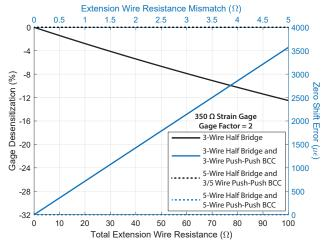
Figure 2. Strain gage desensitization and zero-shift errors
