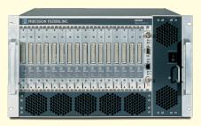
Qty. 4 28016 Mainframes with Power Supplies and 28000F-BIF1-FT Control Cards with Built-In Test Support
