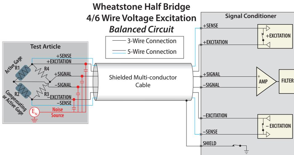
Figure 4. 4/6-wire Wheatstone half bridge with gages and completion resistors collocated
