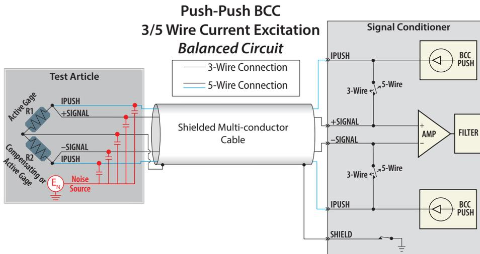
Figure 6. 3/5-wire Push-Push BCC circuit for paired strain gages
