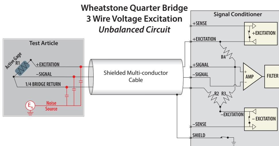
Figure 2. 3-wire Wheatstone quarter bridge circuit
