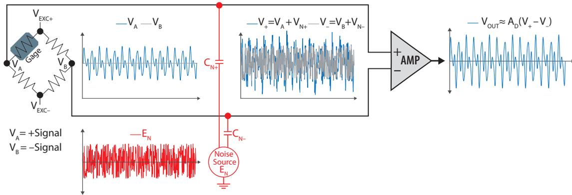
Figure 1. Diagram depicting the basic bridge-based differential circuit used to measure strain
