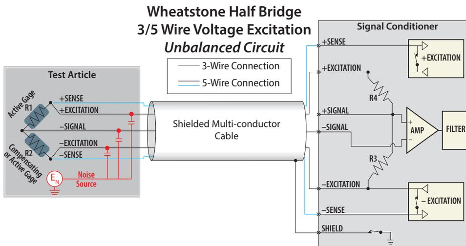
Figure 3. 3/5-wire Wheatstone half bridge circuit
