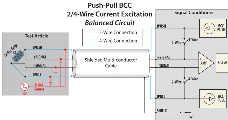
Figure 5. 2/4-wire Push-Pull BCC circuit for a single active strain gage
