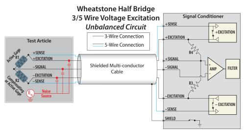
Figure 3. 3/5-wire Wheatstone half bridge circuit
