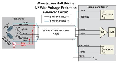
Figure 4. 4/6-wire Wheatstone half bridge with gages and completion resistors collocated
