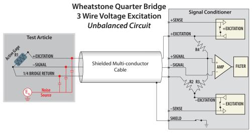
Figure 2. 3-wire Wheatstone quarter bridge circuit
