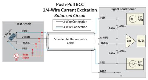
Figure 5. 2/4-wire Push-Pull BCC circuit for a single active strain gage
