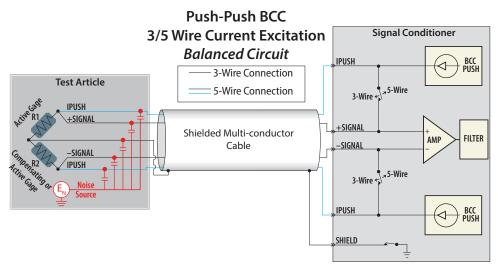
Figure 6. 3/5-wire Push-Push BCC circuit for paired strain gages
