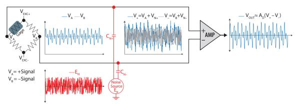
Figure 1. Diagram depicting the basic bridge-based differential circuit used to measure strain
