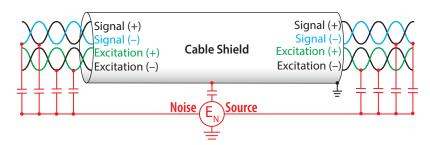
Figure 7. Preferred cable (shielded twisted-pair) for balanced strain gage measurement circuits
