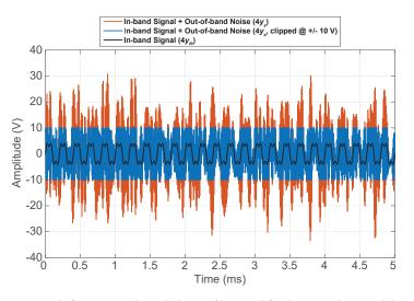
Figure 2. Test signal after passage through the pre-filter amplifier (gain = x4). Beyond the  $\pm 10$  V clipping threshold, the total amplified signal (= 4  $y_s$ ) is clipped and limited to a peak voltage of 10 V. The amplified in-band portion of the signal (= 4  $y_{ib}$ ), which lies below the clipping limits of the amplifier, is shown for reference.
