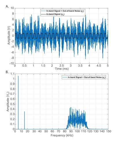
Figure 1. (A) Test signal constructed to demonstrate the effect of invisible clipping. The total signal  $y_s$  includes an in-band component  $y_{ib}$  (peak voltage = 1 V) and out-of-band noise  $y_{ob}$  (rms voltage = 2.4 V). (B) Amplitude spectrum of  $y_s$ . The in-band square wave components  $f_1$  (5 kHz) and  $f_2$  (15 kHz) are clearly distinguishable from the band-limited noise centered at 100 kHz.
