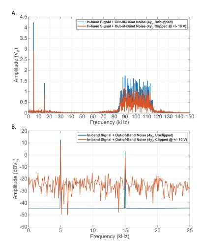
Figure 4. (A) Comparison of amplitude spectra between clipped and unclipped versions of the amplified signal  $y_s$ . (B) Inset from (A) showing the passband of the filter used in this study (LP8P,  $F_c = 25$  kHz) on the decibel scale.
