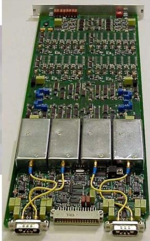
**Figure 9:** Precision Filters, Inc. 28316B 16-Channel IEPE Amplifier/Filter and 28334A 4-Channel Dual Mode Dynamic Charge Conditioner with LDTEDS Capability
