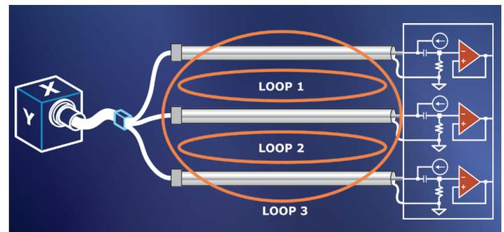
Figure 3: Ground loops created by improper connection of signal conditioner to triaxial accelerometer
