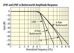
The LP4F and LP8F are a good choice as an anti-aliasing filter and for applications such as spectral analysis. The LP8F has zero passband ripple and over 100 dB/octave attenuation slope.
