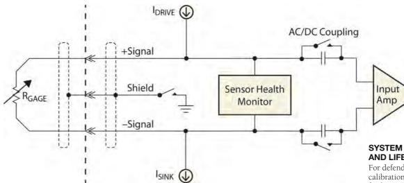
A basic strain gauge cannot distinguish between strain imposed by the mechanical process and expansion of the test material due to its temperature coefficient of expansion. This reporting of strain due to thermal expansion is often called apparent strain.
