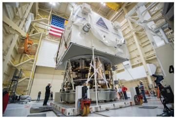
**ESA's European Service Module ready for testing in the Space Power Facility** Courtesy NASA
