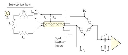
Figure 1: Two-Wire Wheatstone Bridge Connection
