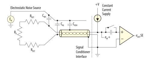
Figure 3: Single-Ended Constant Current Excitation Circuit
