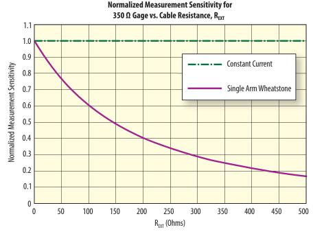
Figure 2: Normalized Measurement Sensitivity vs. R<sub>EXT</sub>
