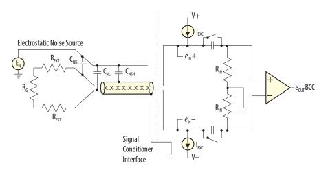
Figure 4: Balanced Constant Current Excitation Circuit
