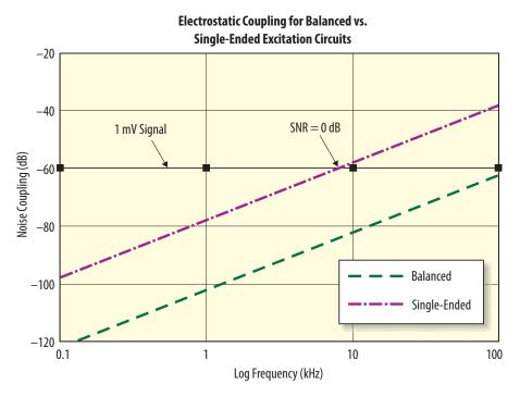
Figure 6: Electrostatic Noise Coupling for Balanced vs. Single-Ended Excitation
