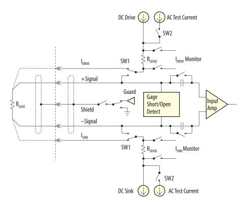
Figure 5: BCC Excitation Circuit Diagram
