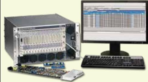
The Precision 28000 system makes it easy to manage a test with hundreds of channels and a mix of transducers. Choose charge, IEPE w/TEDS, voltage (filter amplifier), strain, thermocouple, RTD, potentiometer, current, frequency, or other transducers.
