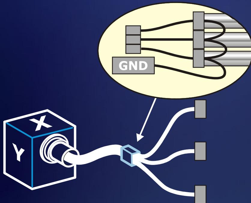
**Note: The shields of each coaxial cable are tied together in the breakout cable**
