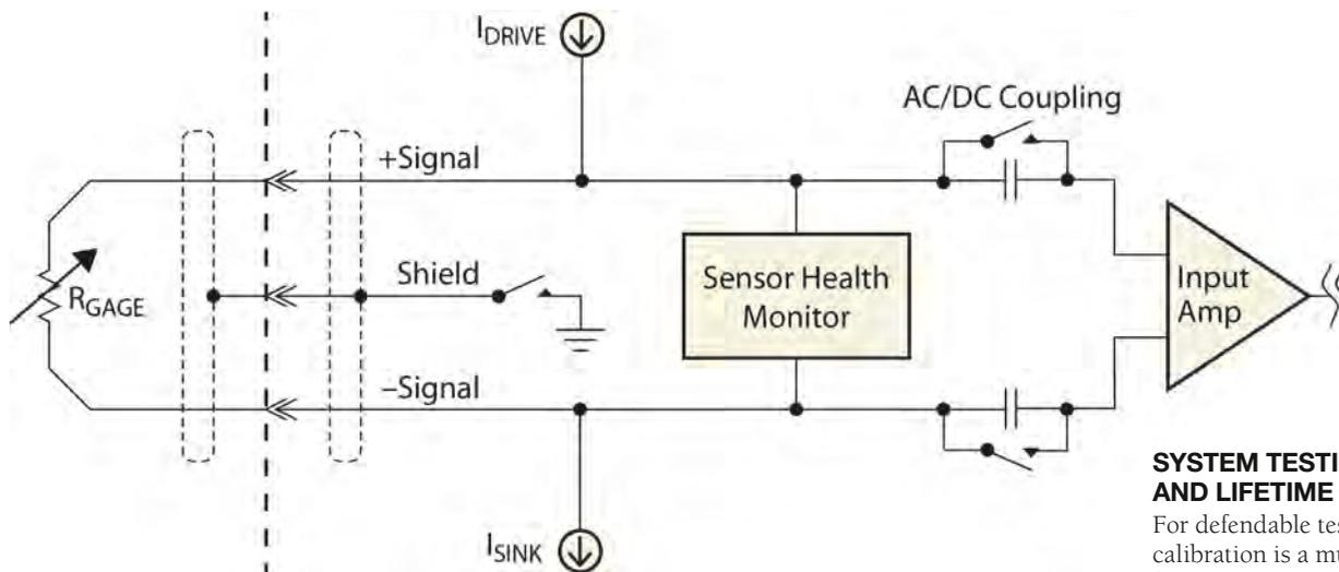
ABOVE: Balanced constant current connection for dynamic strain measurement
